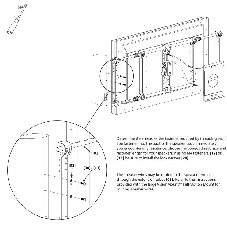
Disconnect the speaker wire from the receiver or amplifier when you route it through the upper or lower extension tubes **[03]** to avoid damage to the speakers, amplifier, or receiver.
